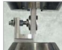
CUTTING RESISTANCE TEST - Ft Ft max = 500 daN (1 daN corresponds approximately to 1 kg weight)
