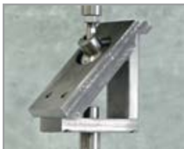
TRACTION RESISTANCE TEST - F F max = 550 daN (1 daN corresponds approximately to 1 kg weight)
