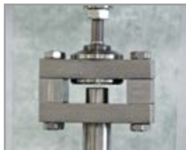
TRACTION RESISTANCE TEST - Fn Fn max = 380 daN (1 daN corresponds approximately to 1 kg weight)
