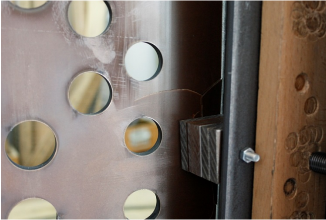
Figure 5: Failure of test assembly no. 101 at the fastening point at the maximum load of 4 kN (interior view)
