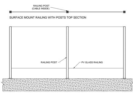
SURFACE MOUNT RAILING WITH POSTS ELEVATION
