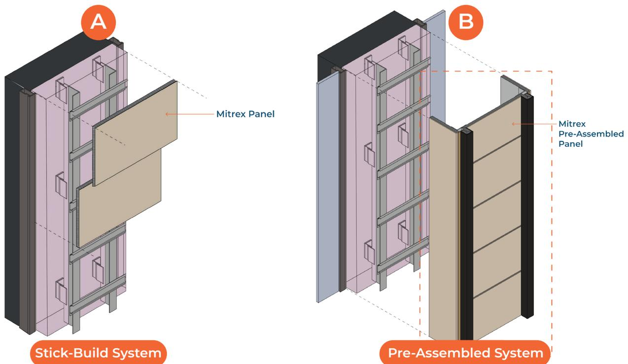
**An air pressurized cavity wall system designed to eliminate water penetration and allow ventilation.**
