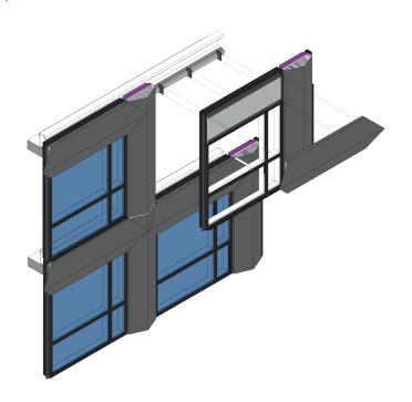
Integration into window walls, curtain walls, mega-panels, modular systems, etc by working with other service providers. This allows for a uniform installation system for the entire building based on prefabricated wall assemblies.
