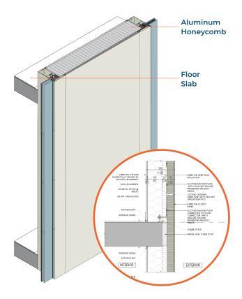
The system is a hybrid of window wall and precast architectural wall panels, spanning slab to slab and transferring all the component loads to the building structure.
