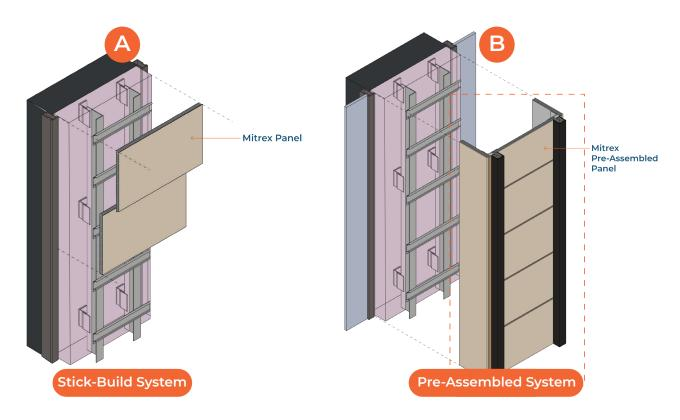
An air pressurized cavity wall system designed to eliminate water penetration and allow ventilation. This system consists of two options: **stick-build cladding** where installation is panel by panel, and **pre-assembled cladding** where the panels are prefabricated and installed as a single unit. This results in faster installation and minimizes connection points to substrate. Panels can span floor to floor and be attached to slabs only.
